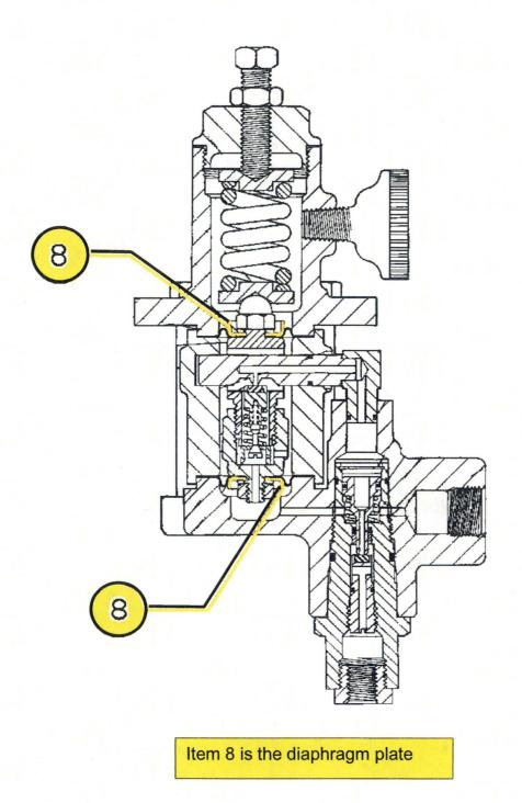
Figure 1: Outline Dwg of Pilot Valve Portion of Regulator Assembly
