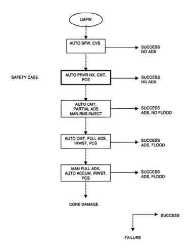
During the recent events, the safeguards actuation was an expected plant response. Successful PRHR and CMT actuation places the plant in a safe stable state without additional operator actions or additional mitigation functions as outlined above (i.e., Success – No ADS).
