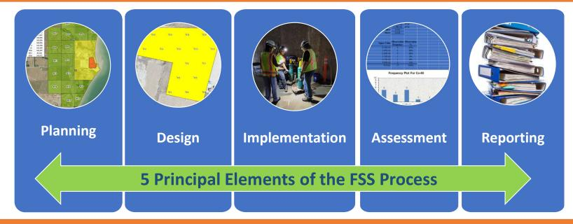
The FSS Plan describes the final radiation survey process used to demonstrate that the site complies with the radiological criteria for unrestricted use specified in 10 CFR 20.1402.
