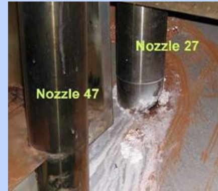
Various Sites Leaking PWR CRDM head penetrations
