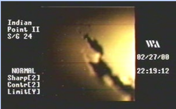
Indian Point (February 2000): SG tube leak hidden by noise in NDE signal
