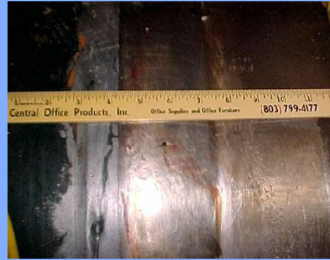
V.C. Summer (Fall 2000): Crack in a hot leg nozzle to pipe weld
