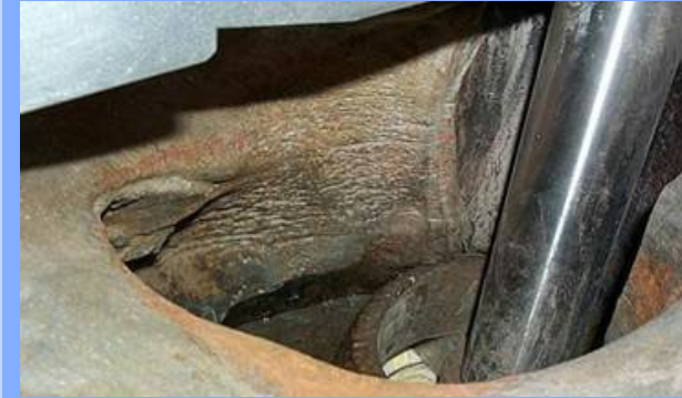
Davis Besse (March 2002): CRDM penetration leakage and head wastage
