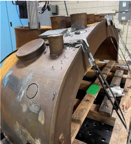
PM-HIP Scaled SMR Head and Valve body
