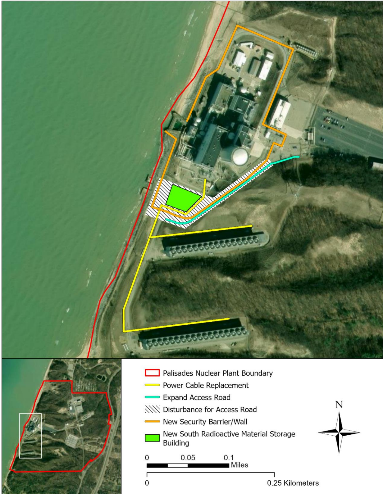
Figure 3-1 Location of Select Ground-Disturbing Activities at Palisades Nuclear Plant Related to the Preparations for the Resumption of Power Operations. Adapted From: HDI 2024-TN10670: RAI-GEN-1.
