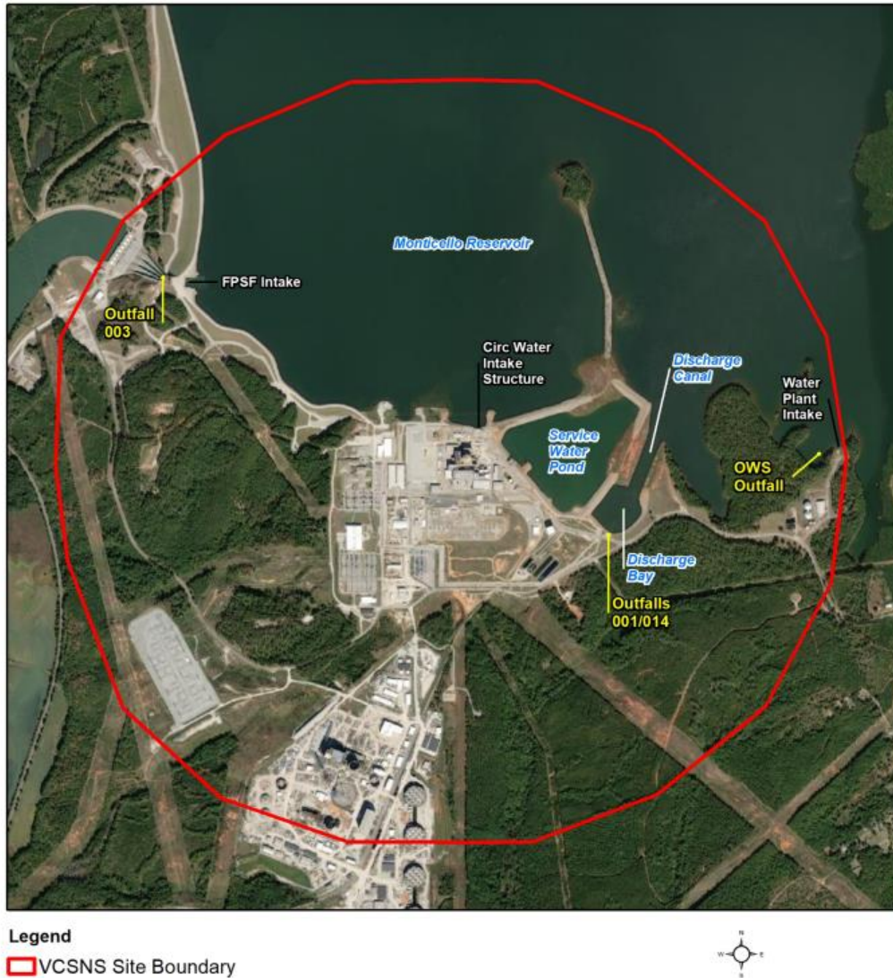
1 2 Figure 3-4 Virgil C. Summer Nuclear Station Site National Pollutant Discharge 3 Elimination System Permitted Outfalls. Source: Dominion 2023-TN10387.
