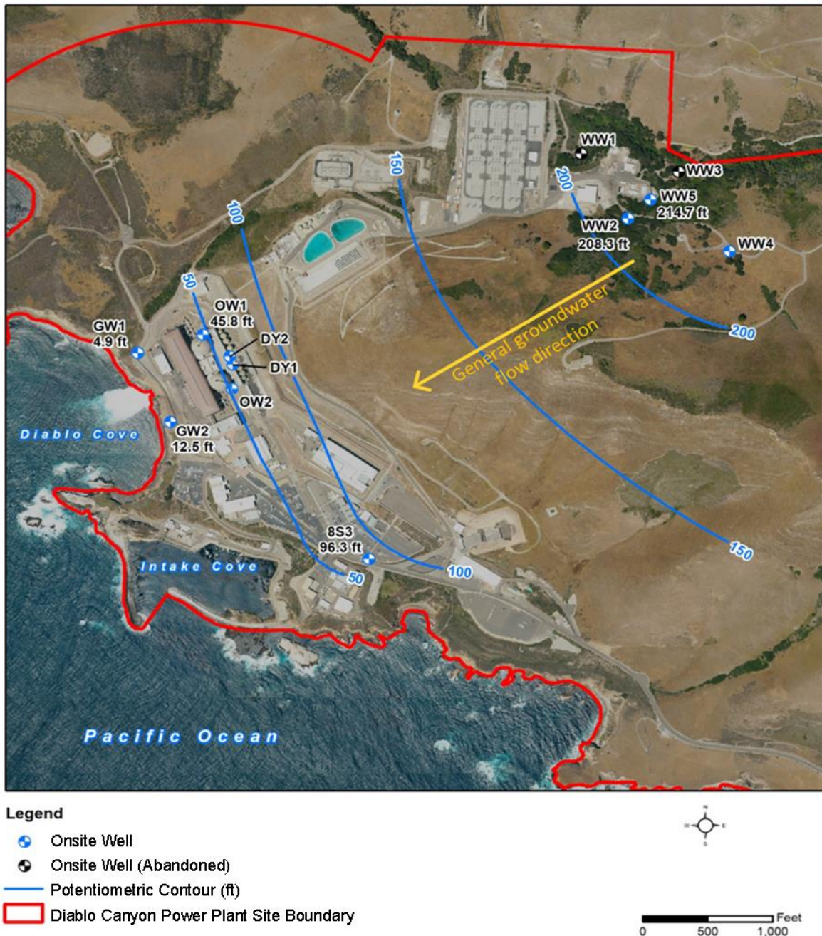
Figure 3-4 Onsite Wells, Estimated Groundwater Levels Based on Data from March 2012, and General Path of Groundwater Flow at the Diablo Canyon Nuclear Power Plant Site. Adapted From ER Figures 3.6-6 and 3.6-7 From PG&E 2023-TN9822.
