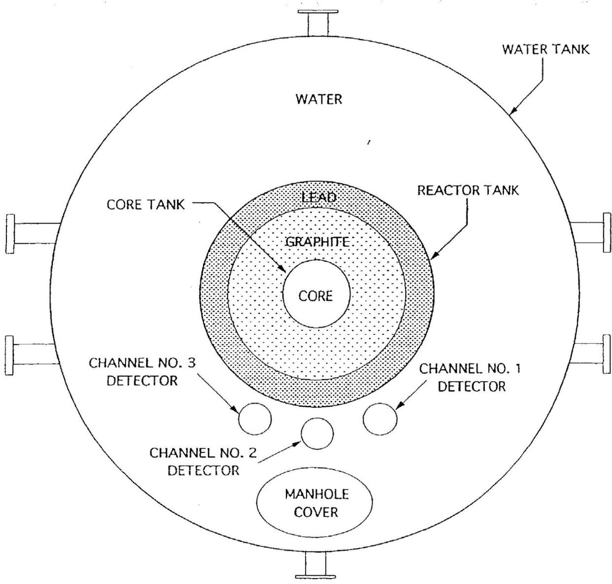
Fig. 4.4-2 Cross section of reactor showing locations of neutron detectors
