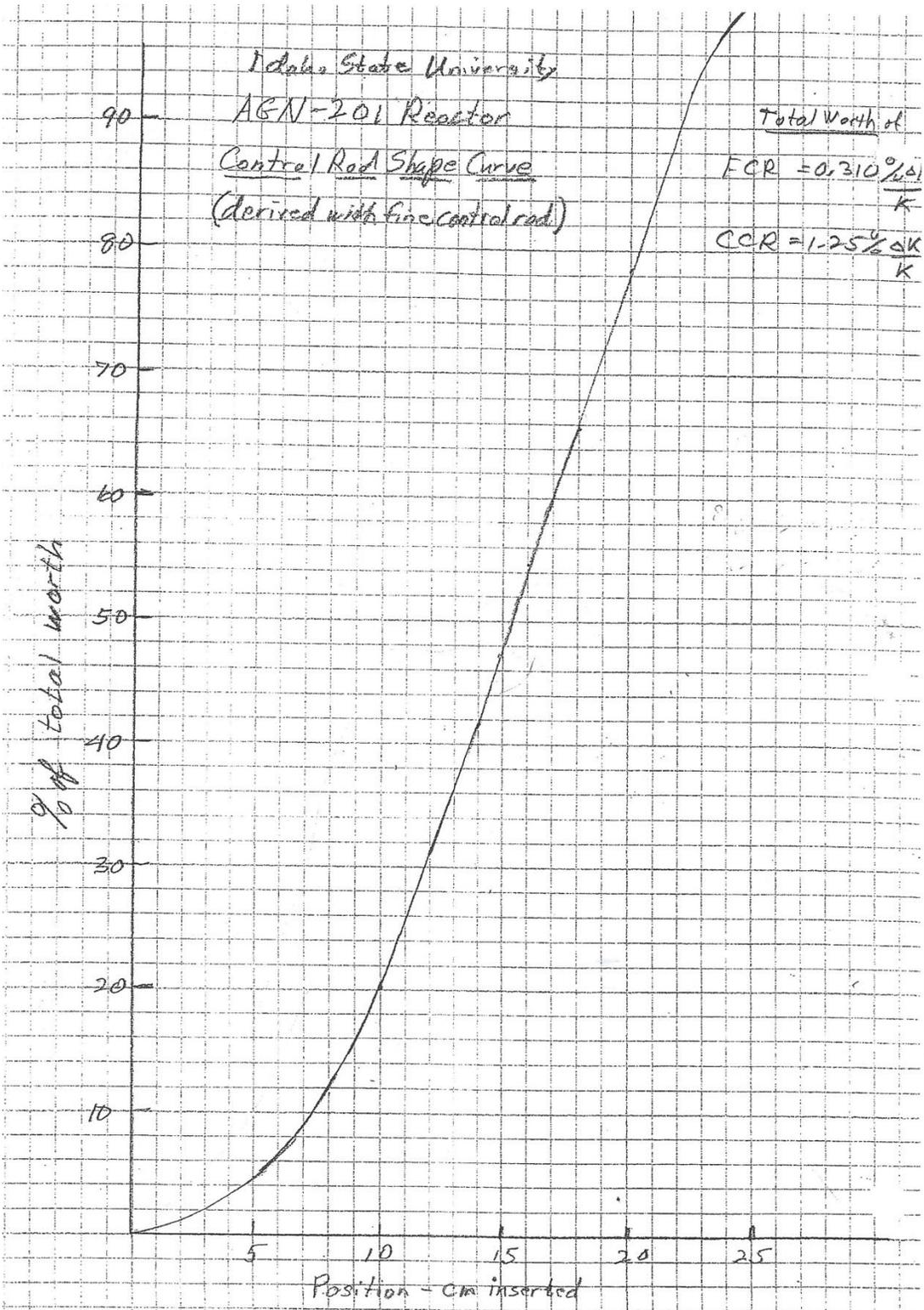
Fig. 4.2-4 Fine Control Rod Calibration Curve
