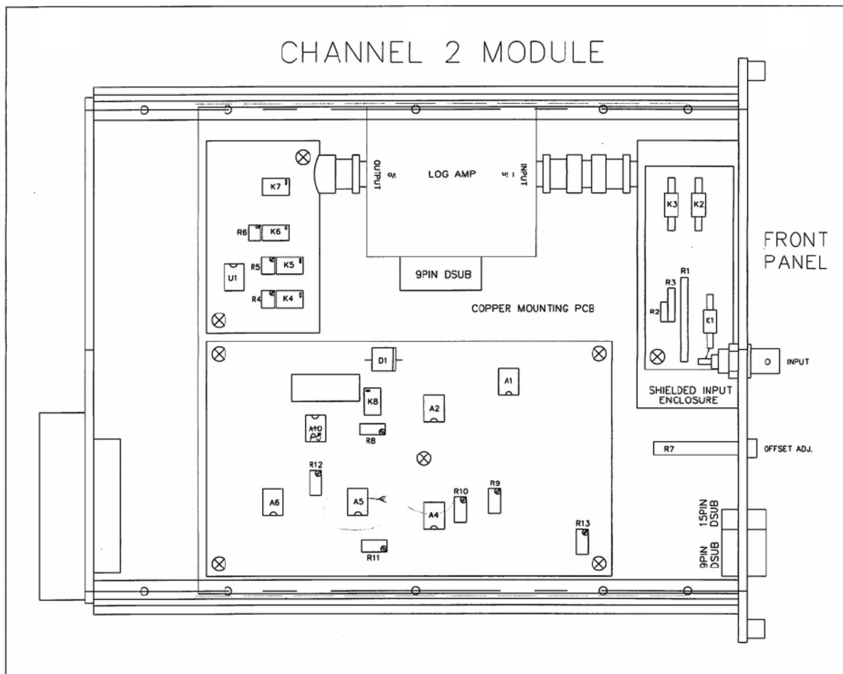
Fig. 4.4-10 Channel 2 Module
