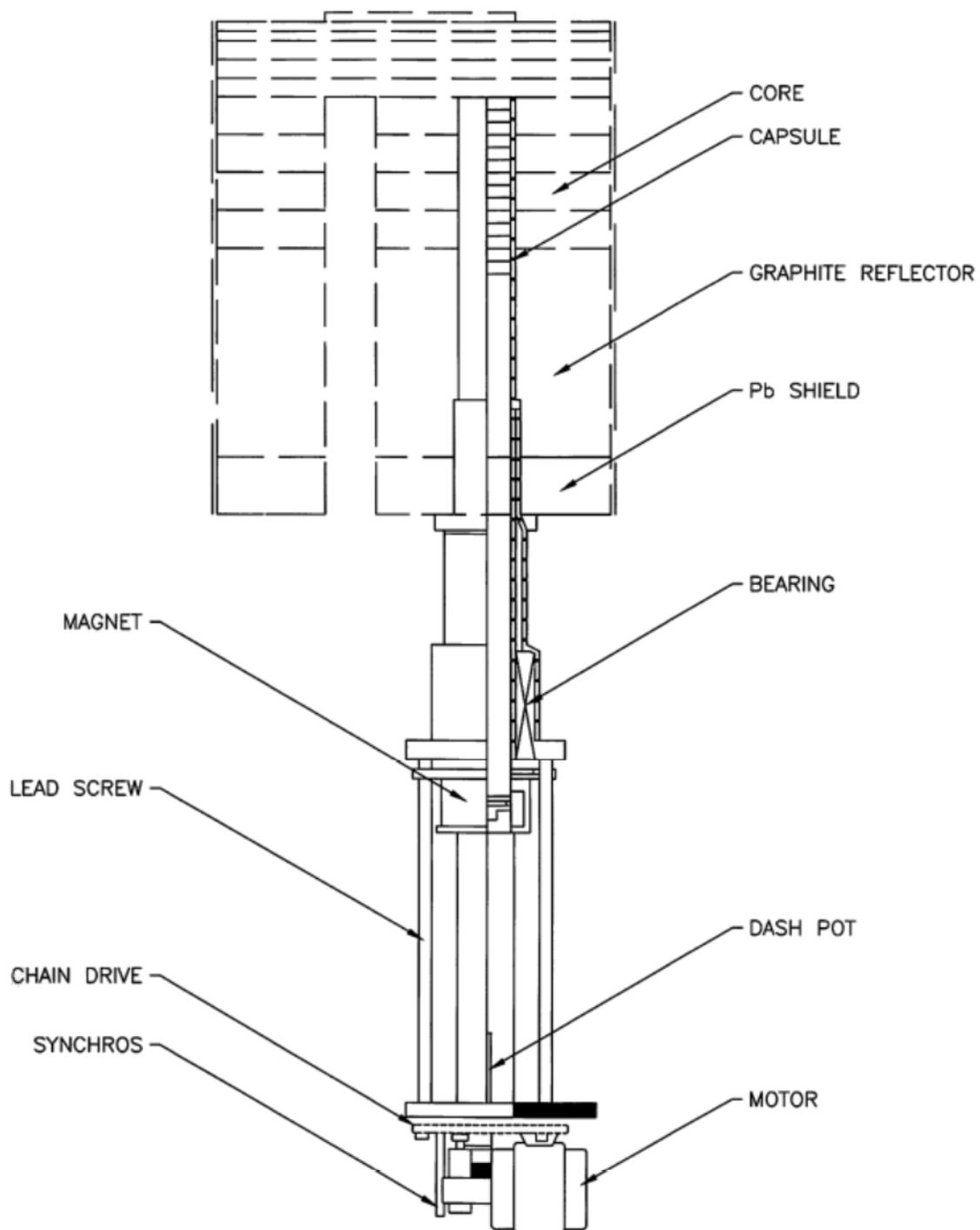
Fig. 4.4-1 AGN-201 control rod and drive mechanism
