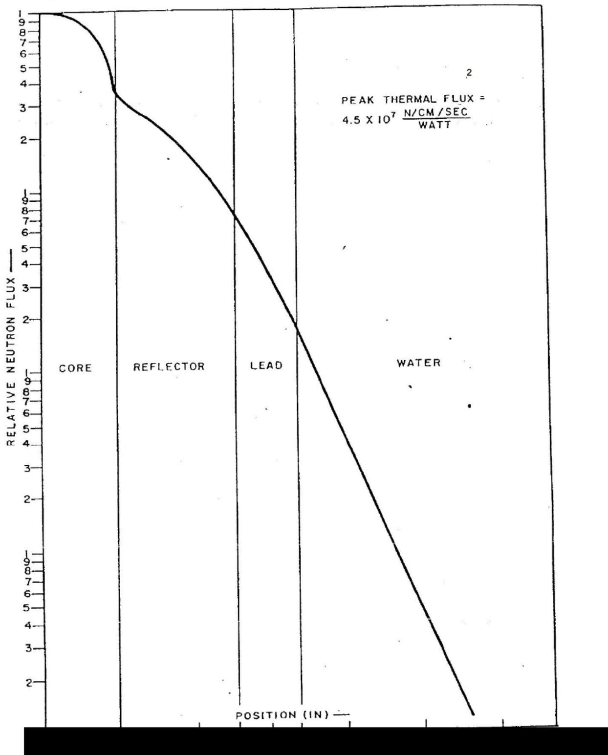
Fig. 4.2-6 Horizontal thermal neutron flux through glory hole at 100 mW
