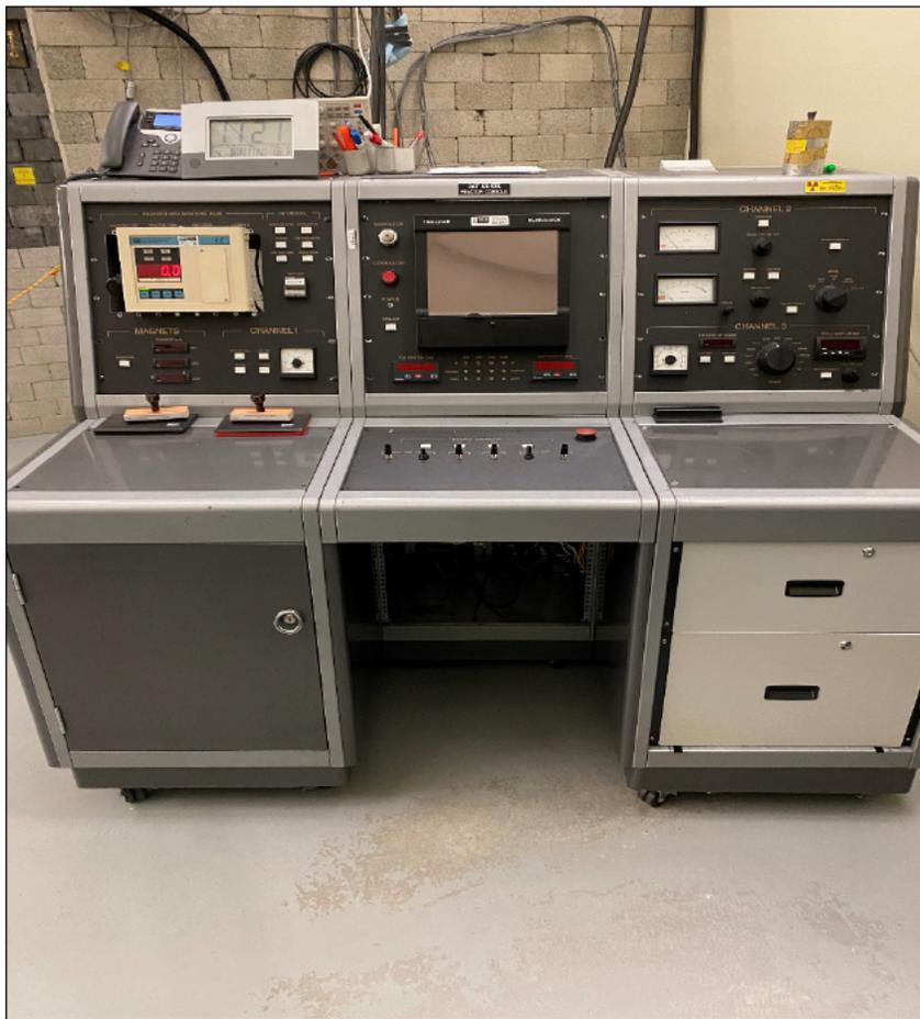
*Fig. 4.2-1 AGN-201 Nuclear Reactor Control console*
