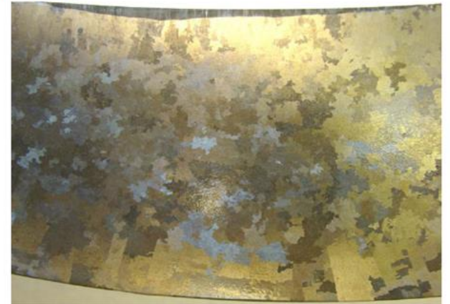
Figure 2-7 Microstructure from 36-in. Specimen Material (vintage material from canceled plant)
