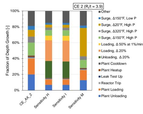
"Representative depth growth" is the average of the total flaw growth divided by the initial quantity of cracks
