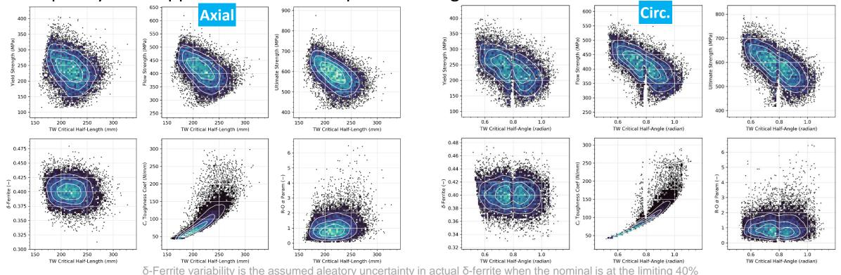
Gap in circumferential point loci due to piecewise-linear equation for psi at  $\pi/4$  and  $\pi/3$  in J-integral calculation (and for dpsi dtheta in dJ/d $\theta$ ) [identical to xLPR equations]
