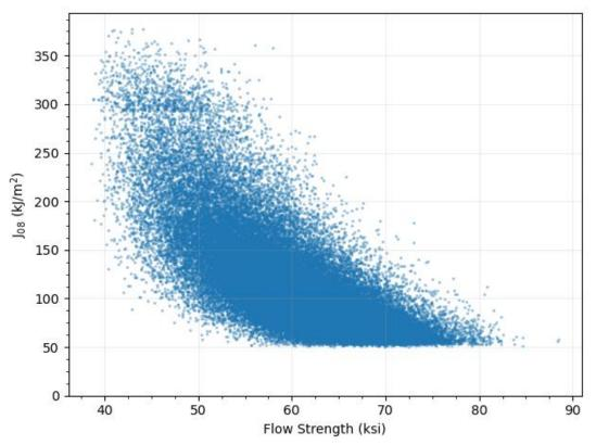
Plot shows data from an example base case PFM run (with 50,000 realizations) for fully aged flow strength and toughness at operating temperature with 40%  $\delta$ -ferrite
