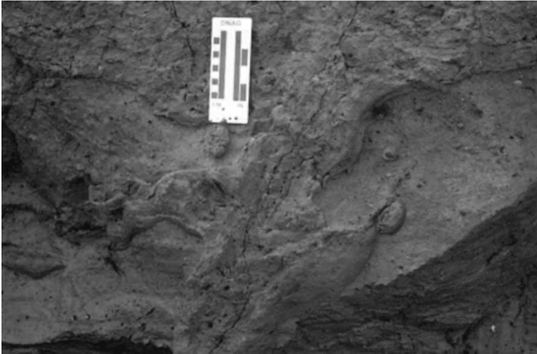
Figure 7, Ashtabula glacial till with oxidized secondary fractures from Bruno, Szabo and Foos, 2006. Source: https://kb.osu.edu/search?query=April%202006&scope=26dee3b3-05fb-57ce-9059-eb615033b352&spc.page=1
