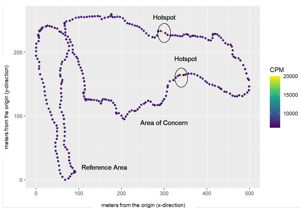
Figure A.5. Data set 2 visualization of radiation measurements (in CPM) across a land area with a reference area and area of concern with two hot spots.
