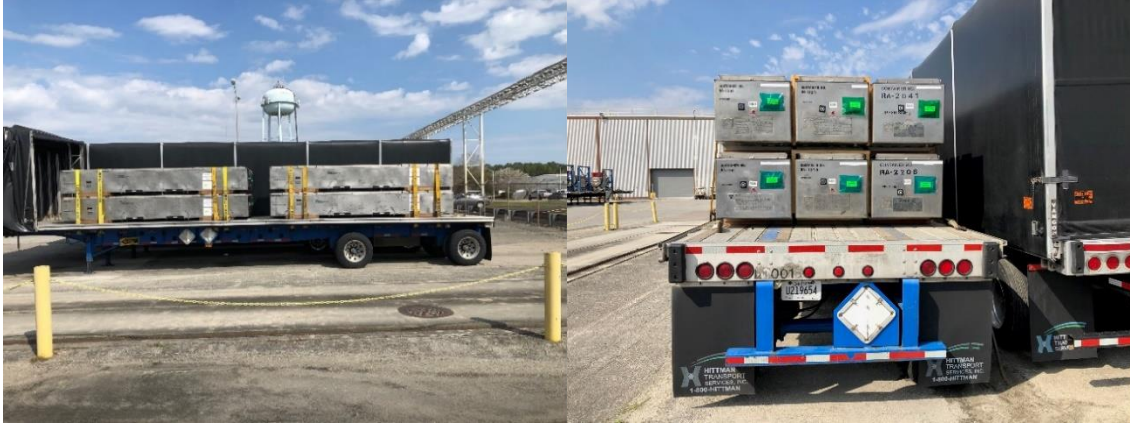
1 2 Figure 3-8 Unirradiated Boiling Water Reactor Fuel Shipment Using RAJ-II Packages. 3 (Photos courtesy of Global Nuclear Fuels, General Electric)
