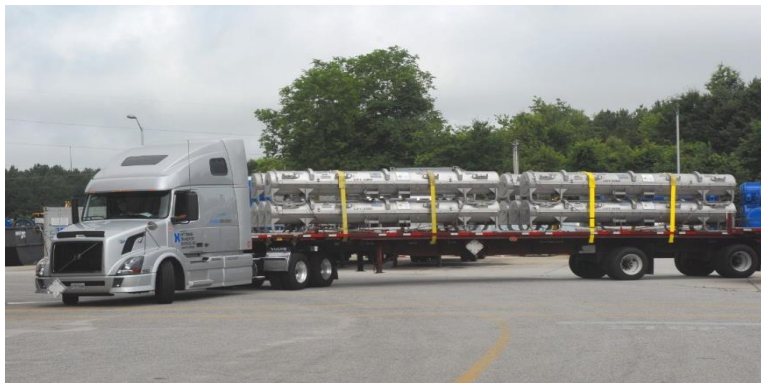
26 27 Figure 3-7 Unirradiated Pressurized Water Reactor Fuel Shipment Using Tc. (Source: 28 Photo provided by the Westinghouse Electric Company, LLC [NRC 2022- 29 TN8089])
