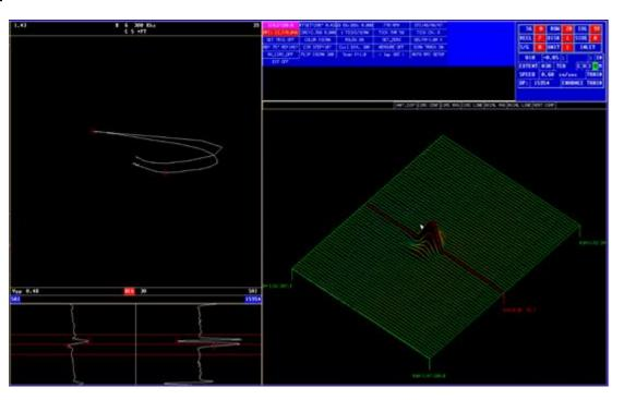
Post crack condition more resembles PWSCC than ODSCC due to phase suppression by the residual. The larger the ding, the greater the phase suppression of flaw signal
