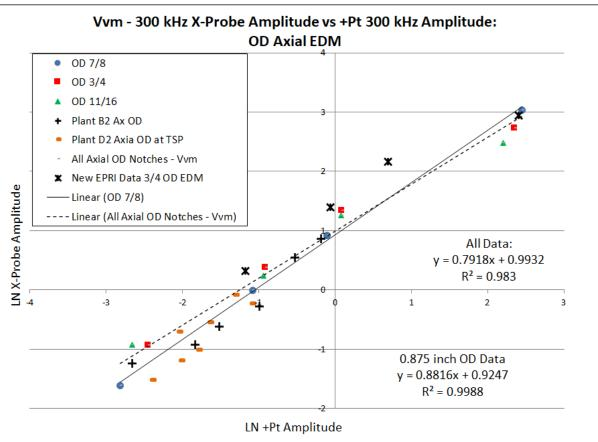
Vpp performance is similar, Vvm shown here since Vvm is used for A-hat development. Volumetric degradation follows the axial ODSCC trending.
