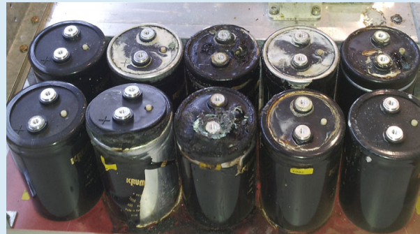
Failed capacitor bank – end of life failures
