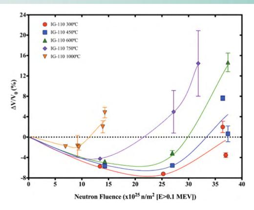
Dimensional change is in general orthotropic. Degree of orthotropy varies with irradiation temperature.
