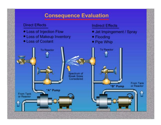
The goal of the consequence evaluation is to assigned a consequence rank (High, Medium or Low) to the piping segment under evaluation.
