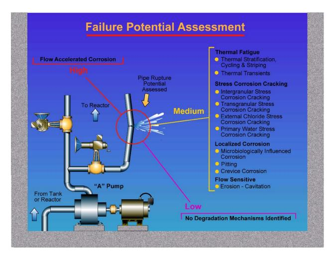
The goal of the degradation mechanism evaluation is to assigned a failure potential rank (High, Medium or Low) to the piping segment under evaluation.
