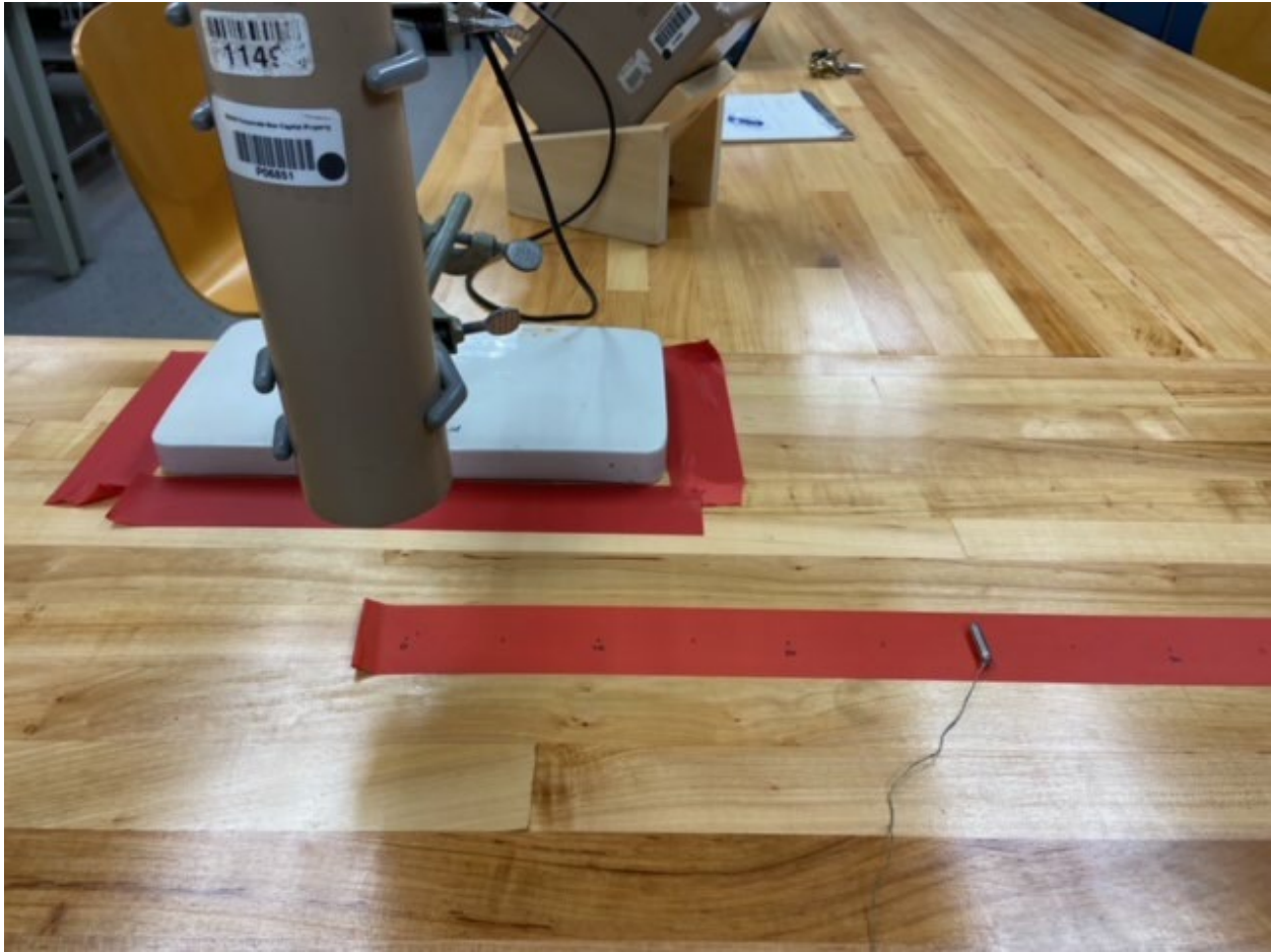
Figure 3.5. Offset experiment using a 4.76 \mu\text{Ci} Co-60 source
