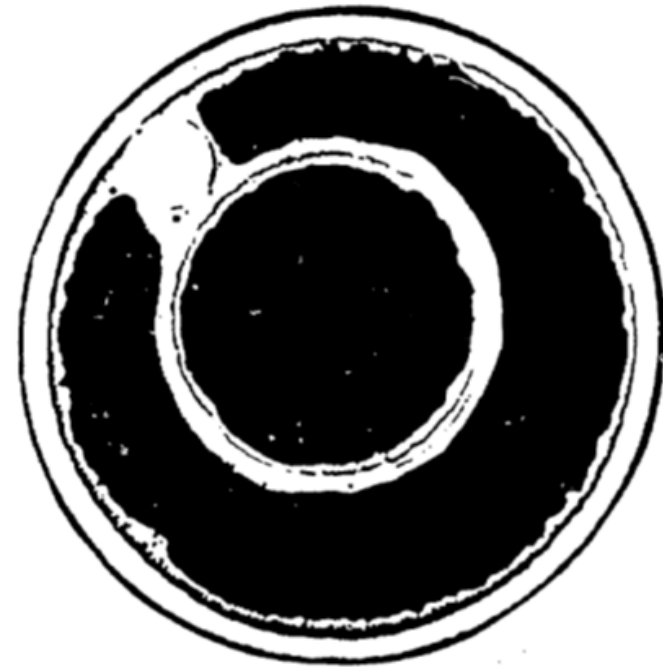
Partial flow blockage from fuel that had been expelled from the cladding and subsequently re-solidified
