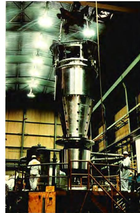
Prototype sodium pump internals
