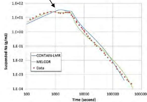
Figure 33. Suspended Na Aerosol Mass - AB1
