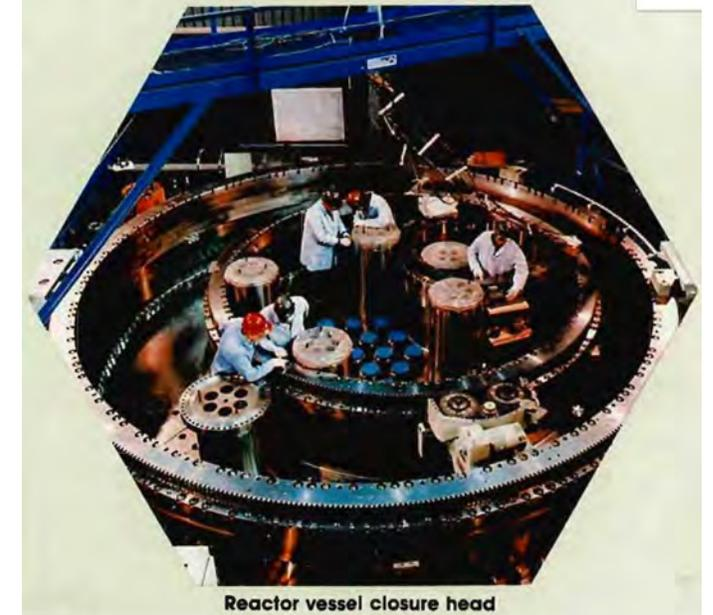
Reactor vessel closure head
