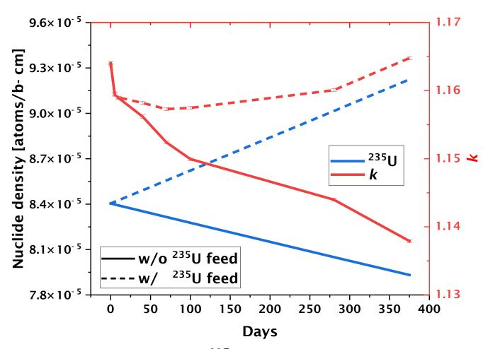
Comparison of <sup>235</sup>U nuclide densities and eigenvalue with and without <sup>235</sup>U feed
