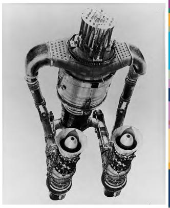
Heat Transfer Reactor Experiment #3
