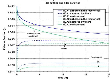
Note: The capture efficiency of the absolute filters for aerosols below <0.3  $\mu m$  was assumed to be zero.
