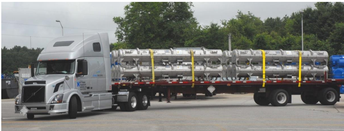
Figure 3-26 Ten Traveller Unirradiated Fuel Transportation Packages Being Transported on a Truck (Source: Photo provided by the WEC)
