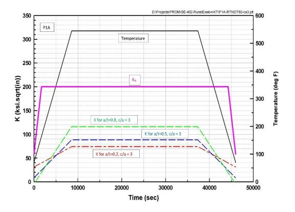
Figure RAI 6-1: Applied K vs. Fracture Toughness as a Function of Temperature for Case ID SGPNV-P1A-(N) (Using Braidwood Unit 2 and Byron Unit 2 Plant-Specific Upper Bound SG Material RTNDT Value of 60°F)
