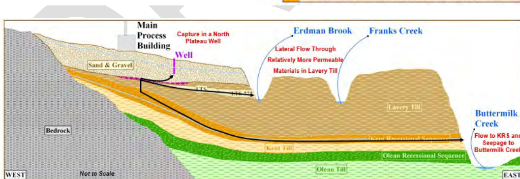
Figure 2 Cross Section Showing Potential Pathways of Exposure Through Ground and Surface Water
