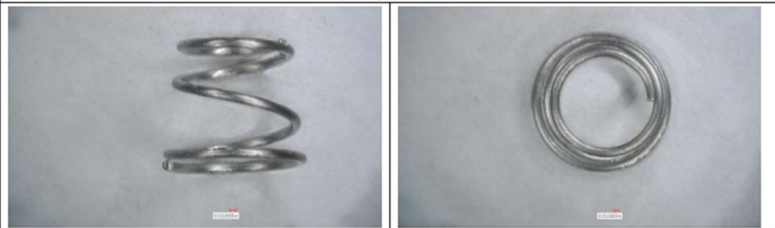
Photos 3 & 4 – Typical Contact Carrier Spring
