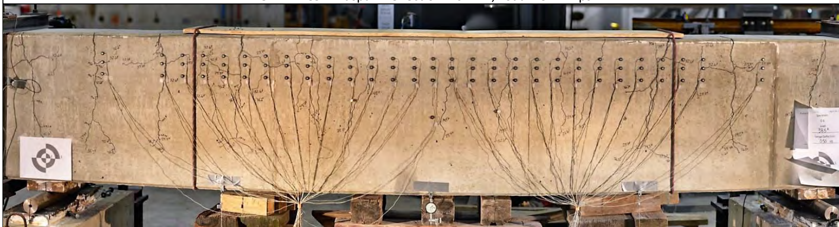
GIRDER C5: Midspan Deflection = 0.4 in., Load = 37.2 kips
