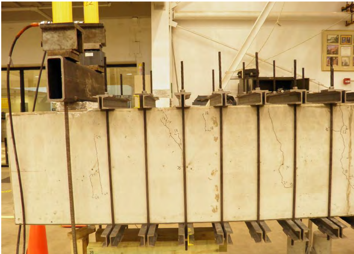
Figure 5 Photograph of One of The Cantilevered Segments of A Test Girder
