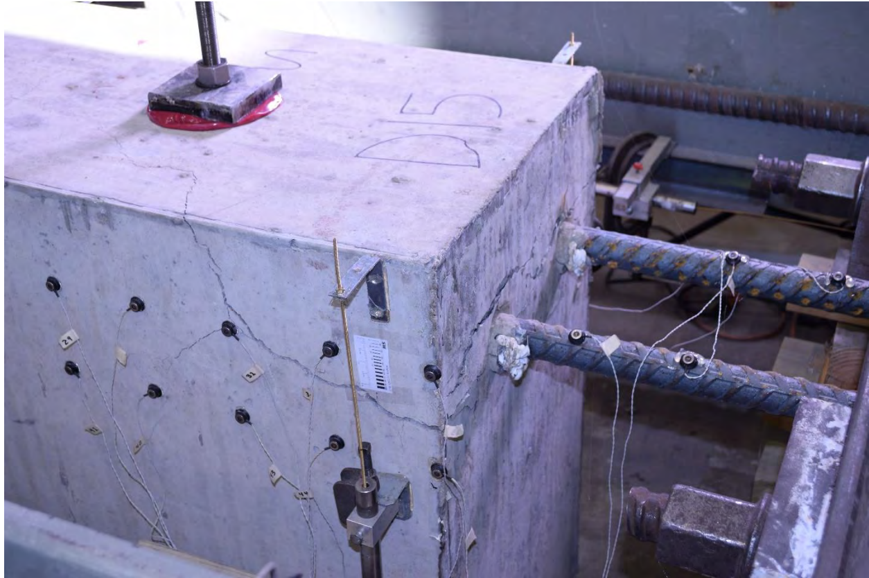
Figure 96 Test Photo Specimen D15, SW corner, 120 kips
