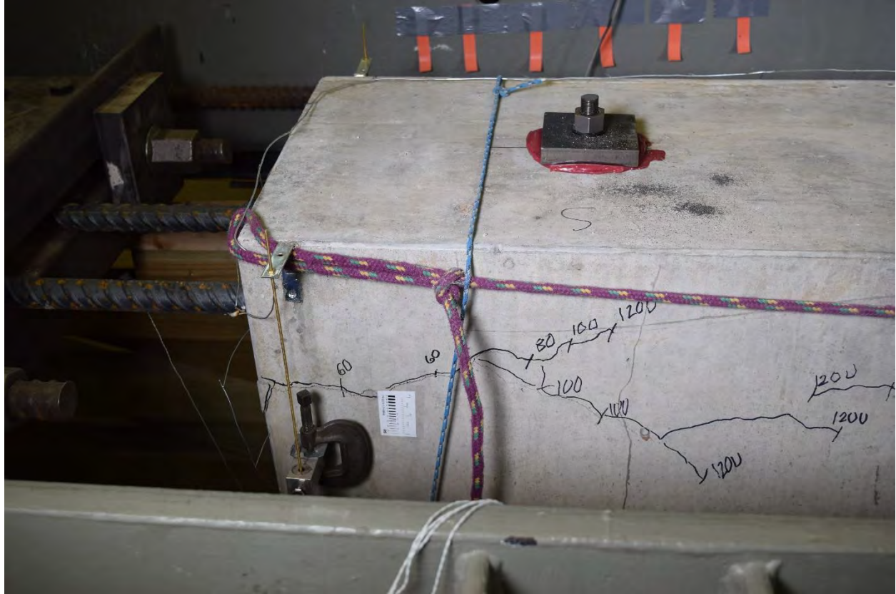
Figure 89 Test Photo Specimen D8, SE corner, 126 kips
