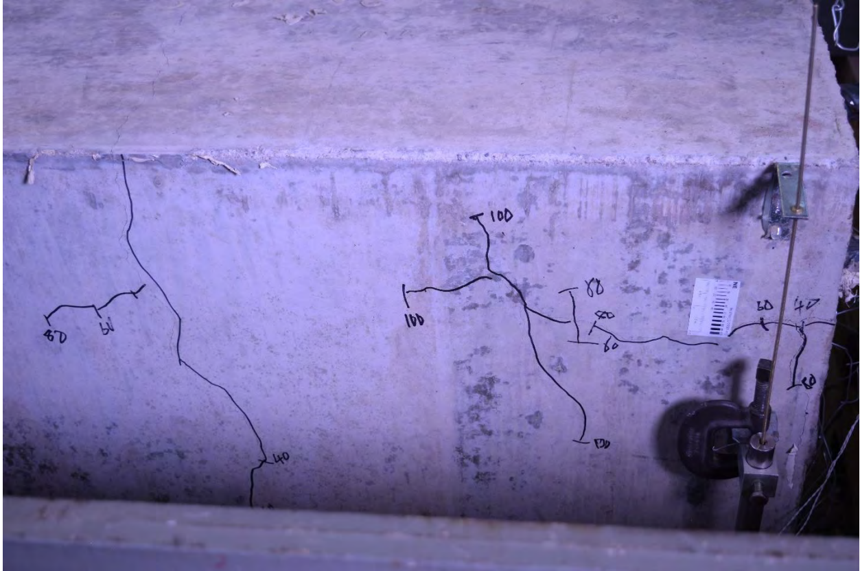
Figure 98 Test Photo Specimen D17, NE corner, 110 kips
