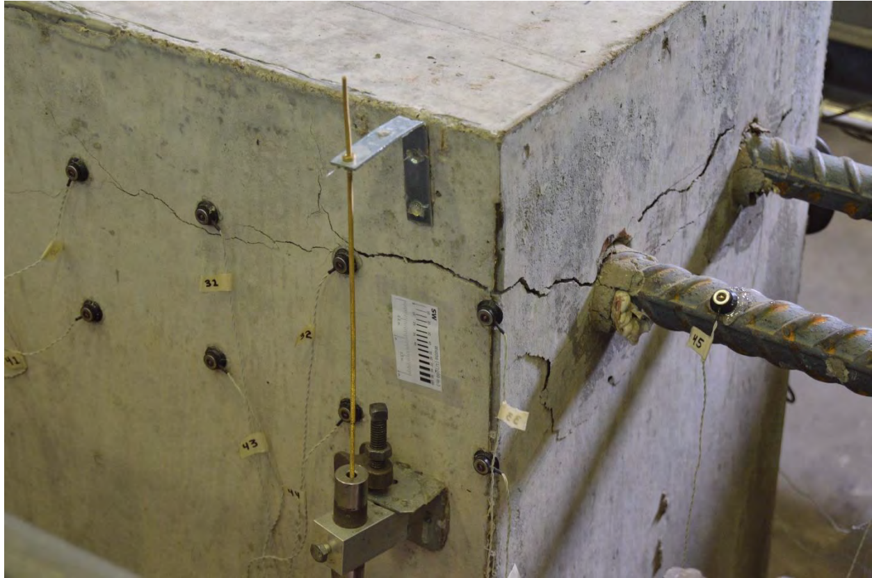
Figure 94 Test Photo Specimen D13, SW corner, 120 kips
