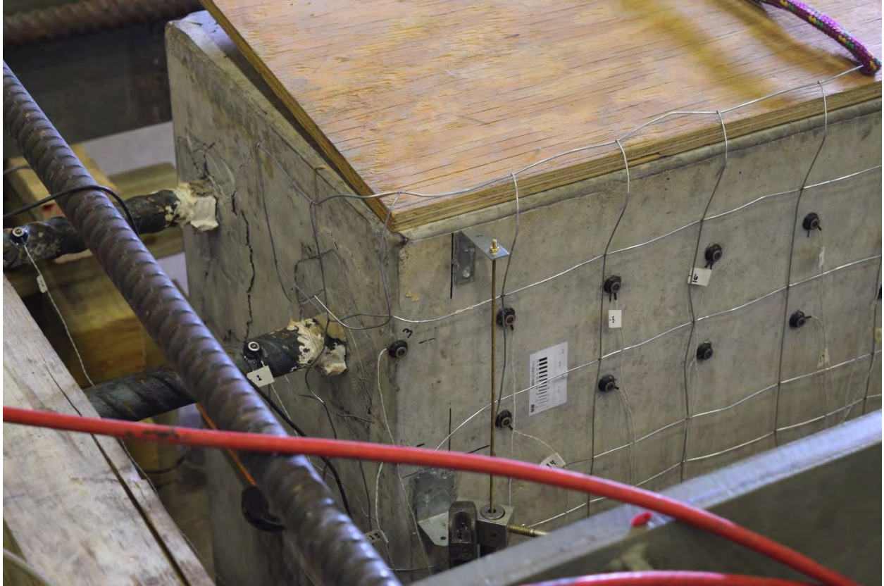
Figure 85 Test Photo Specimen D4, NW corner, 122 kips
