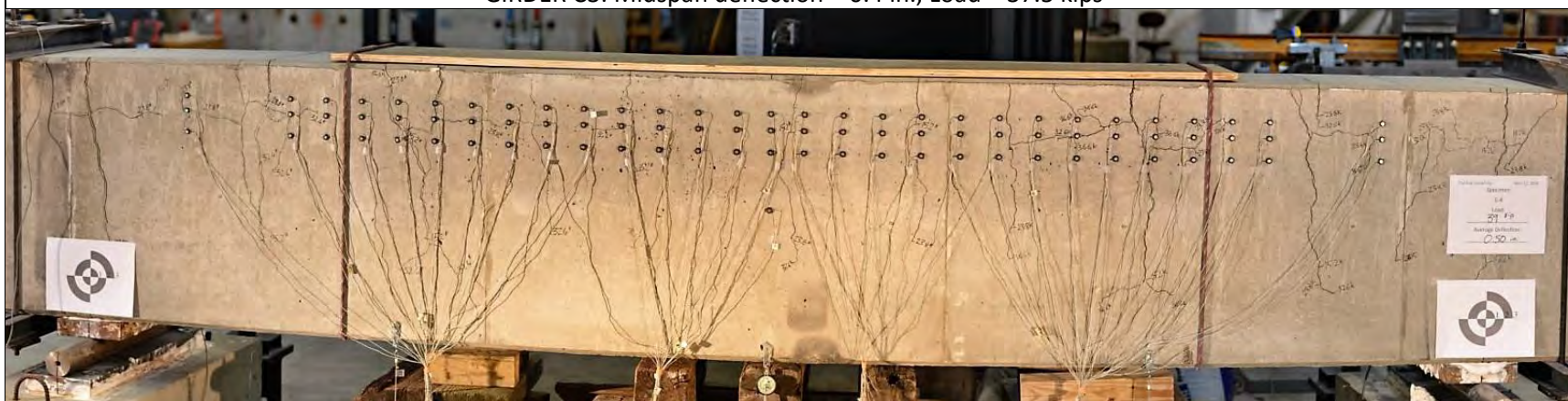
GIRDER C3: Midspan deflection = 0.4 in., Load = 37.5 kips
