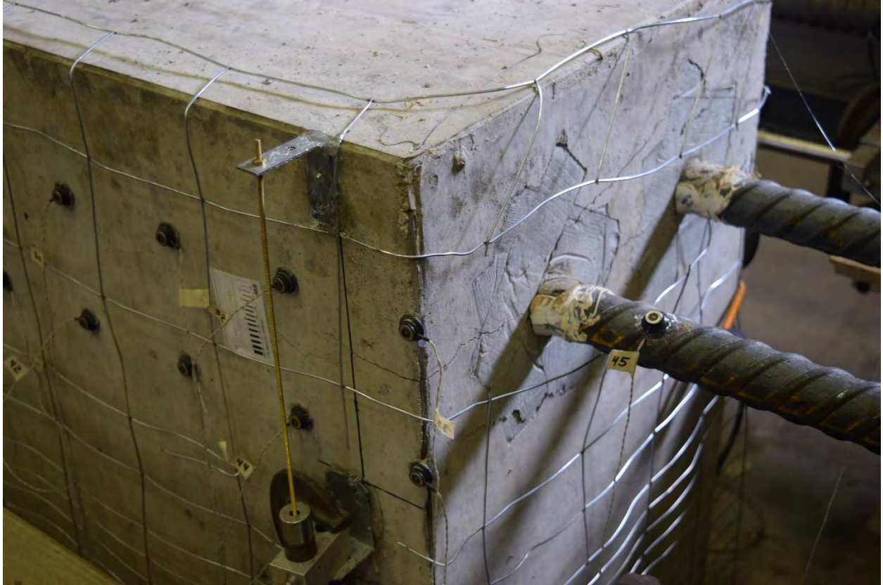
Figure 87 Test Photo Specimen D6, SW corner, 110 kips
