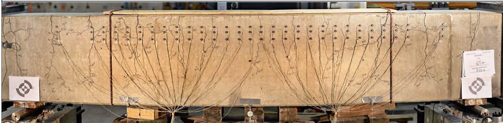
GIRDER C5: Midspan deflection = 0.4 in., Load = 35.1 kips
