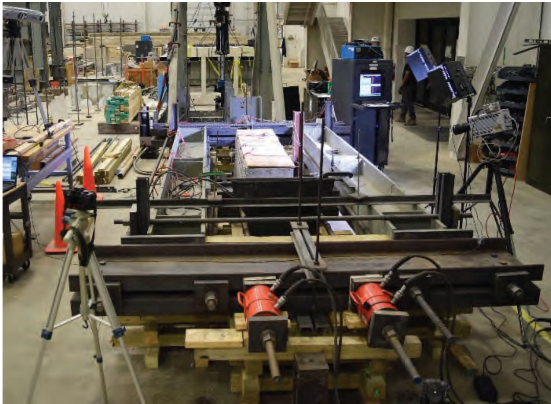
Figure 17: Series D Test Setup and Loading Arrangement (From Ref. 1c)
