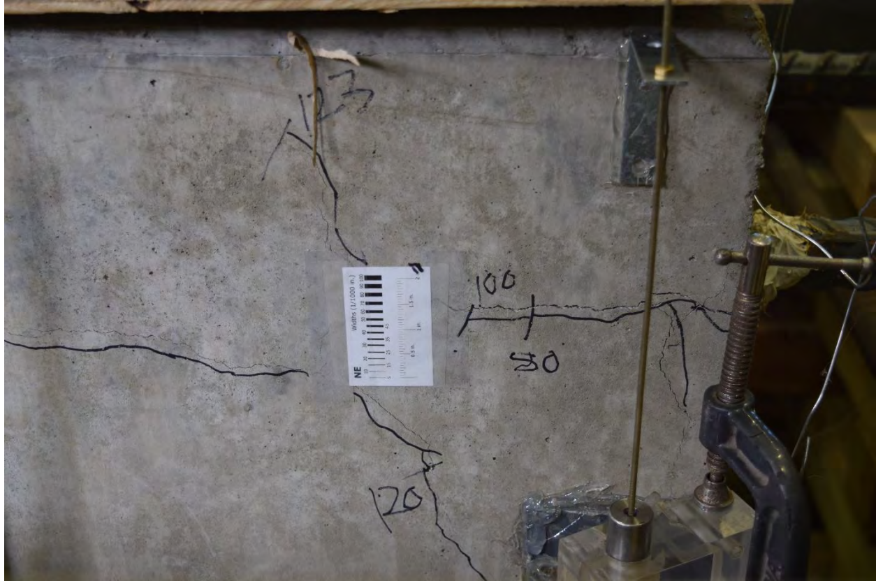
Figure 83 Test Photo Specimen D2, NE corner, 90 kips
