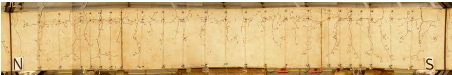
Figure 9 West Elevation of Test Girder A4 Reloaded to 36 kip
