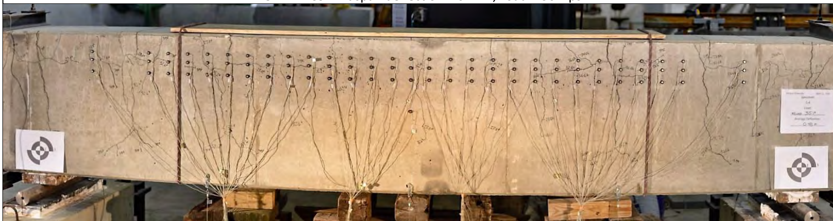
GIRDER C3: Midspan deflection = 0.4 in., Load = 36 kips
