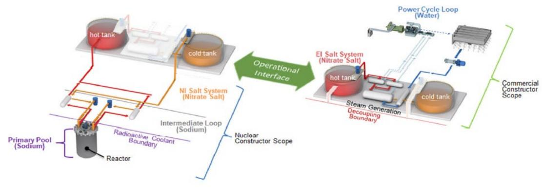
Molten salt storage tanks eliminate direct coupling of reactor power and turbine output that are inherent in PWR and BWRs
