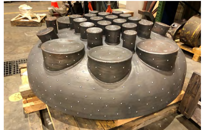
Powder Metallurgy-HIP: 100-10,000 lbs (45-4500 kg)
