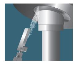
Water-jet and laser peening provide improved surface stresses to mitigate against SCC
