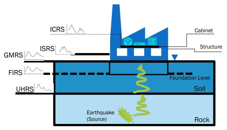
IHRS: Uniform Hazard Response Spectra GMRS: Ground Motion Response Spectra FIRS: Foundation Input Response Spectra ISRS: In-Structure Response Spectra ICRS: In-Cabinet Response Spectra
