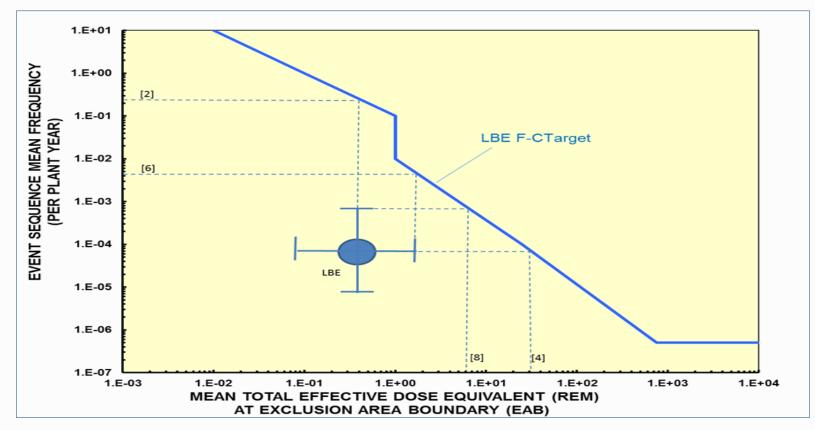
Seismic RIPB for LMP
