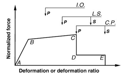
(c) Component or element deformation limits
