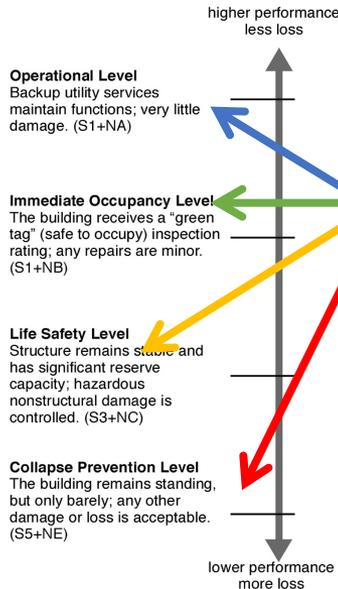
Table 1-2. Deformation and Damage by Limit State.
