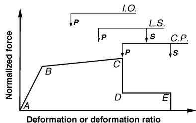
(c) Component or element deformation limits
