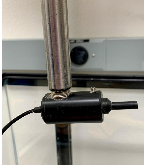
Figure 4.6. The pencil probe used in this study. The probe is housed within a sleeve, which is mounted inside a holder that can be attached to the scanning arm.
