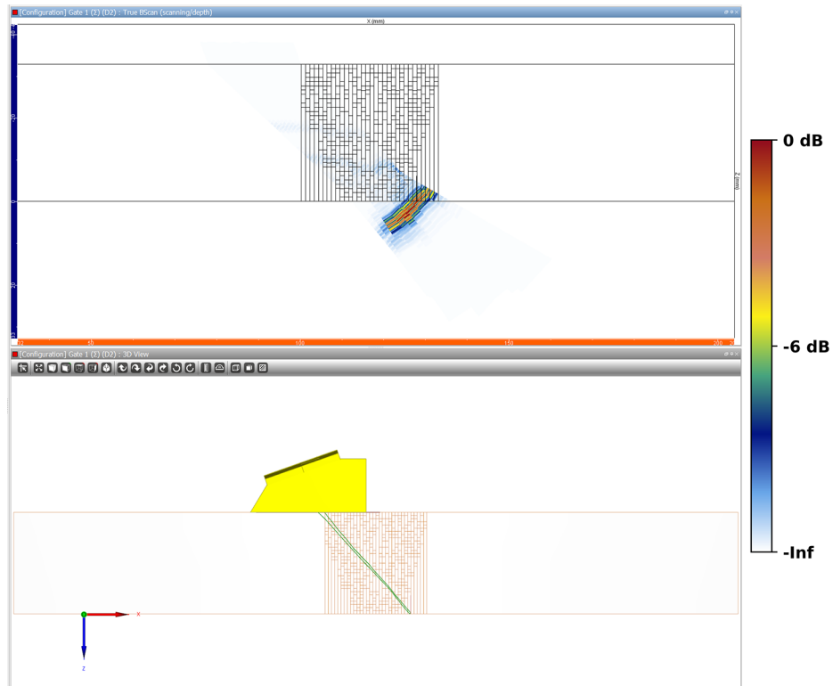
Figure 5.53. Flaw response simulation through the austenitic weld model using the 2 MHz TRL probe at 45^\circ with no interface interactions. The green line is the transmitted and reflected beam.
