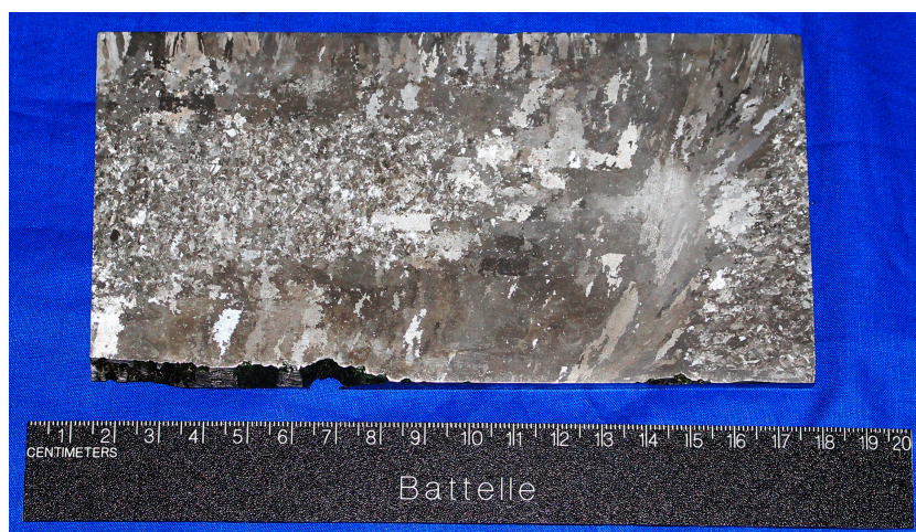
Figure 7.27. A polished and etched circumferential section of a CASS specimen. This figure illustrates that a large variety of grain sizes can exist in the same section.
