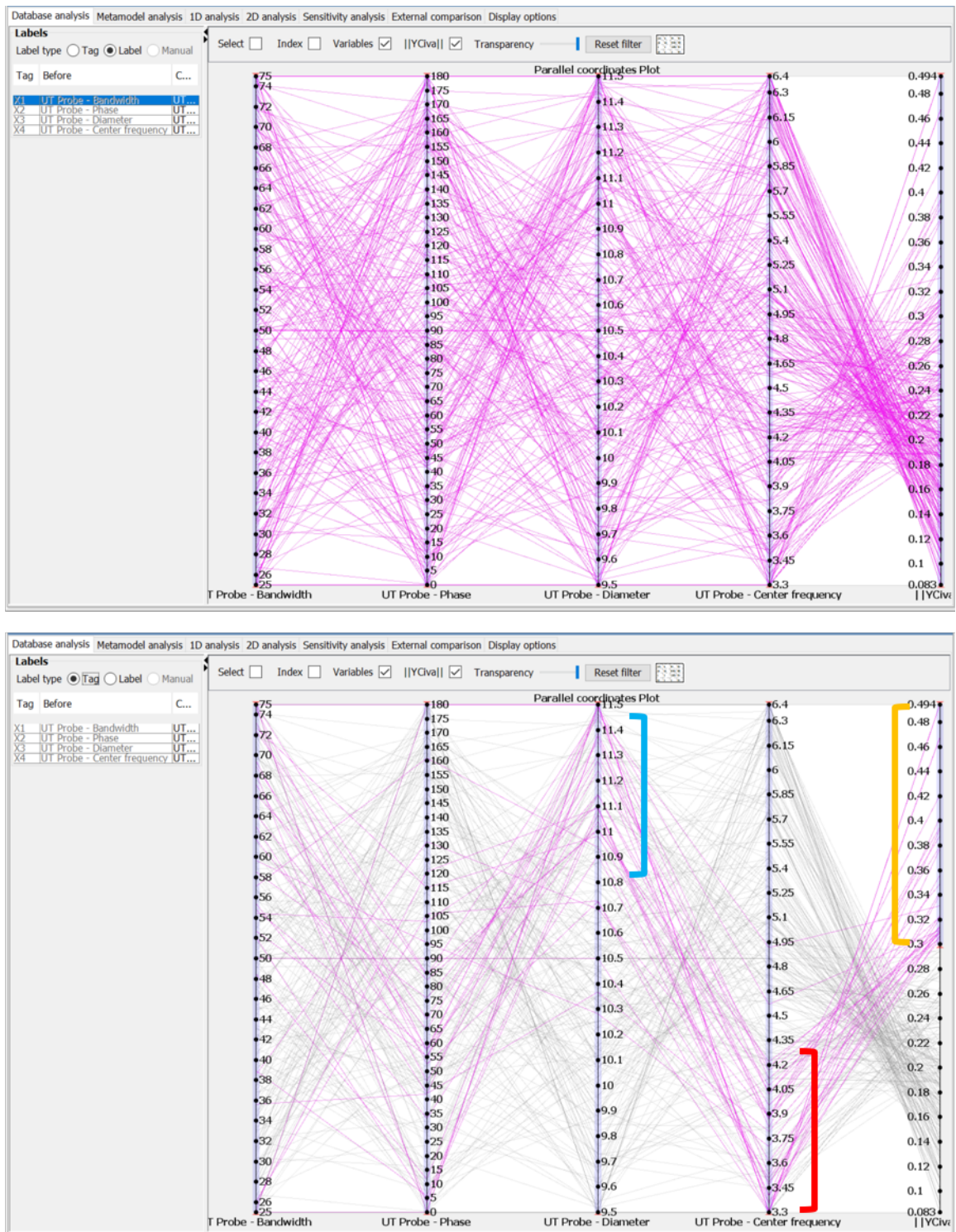
Figure 3.6. Parallel plot showing the relationships between the different variation parameters. Top: Unfiltered plot. Bottom: Plot with a filter applied to the output values such that the highest output values are highlighted (yellow bracket). The filter reveals that the lowest values of probe center frequency (red bracket) combined with the highest values of probe diameter (blue bracket) generally resulted in the highest output values.
