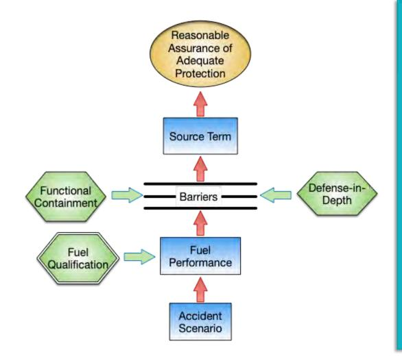
Fuel qualification is a process which provides high confidence that physical and chemical behavior of fuel is sufficiently understood so that it can be adequately modeled for both normal and accident conditions, reflecting the role of the fuel design in the overall safety of the facility. Uncertainties are defined so that calculated fission product releases include the appropriate margins to ensure conservative calculation of radiological dose consequences. -ML17220A315
