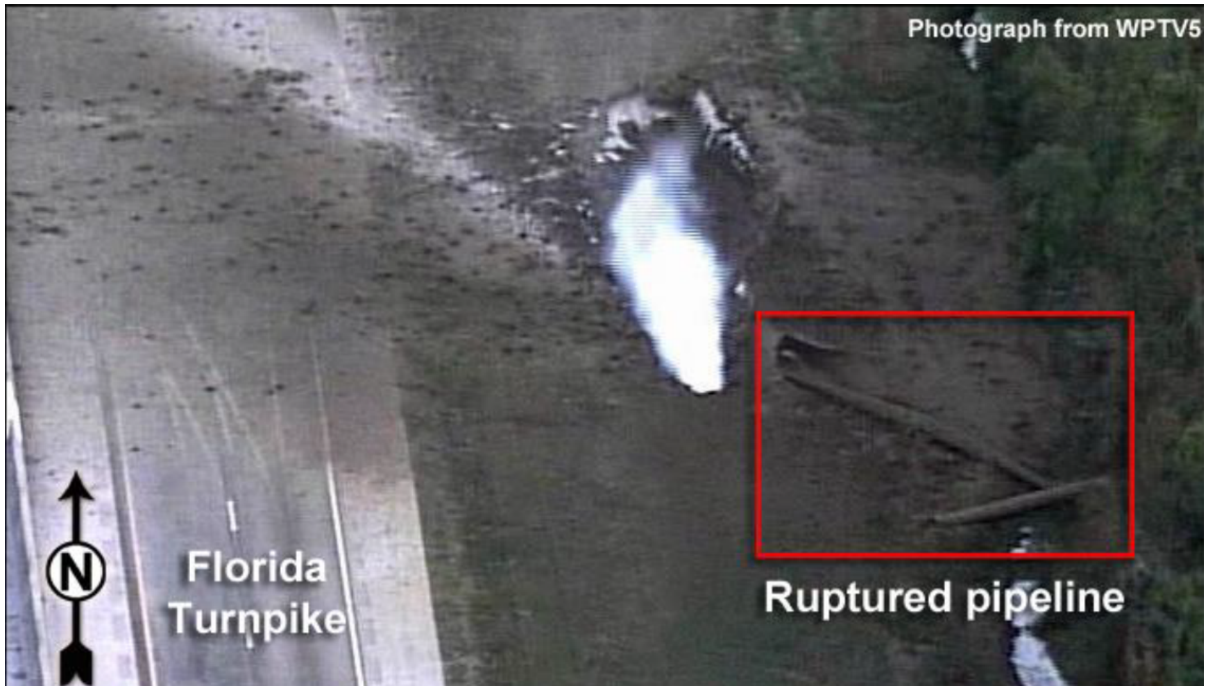
Figure 7. Aerial image of a dense methane cloud from a National Transportation Safety Board report. 208
