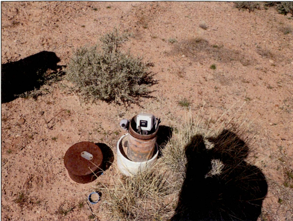
PL-13. Datalogger in Monitoring Well 0906
