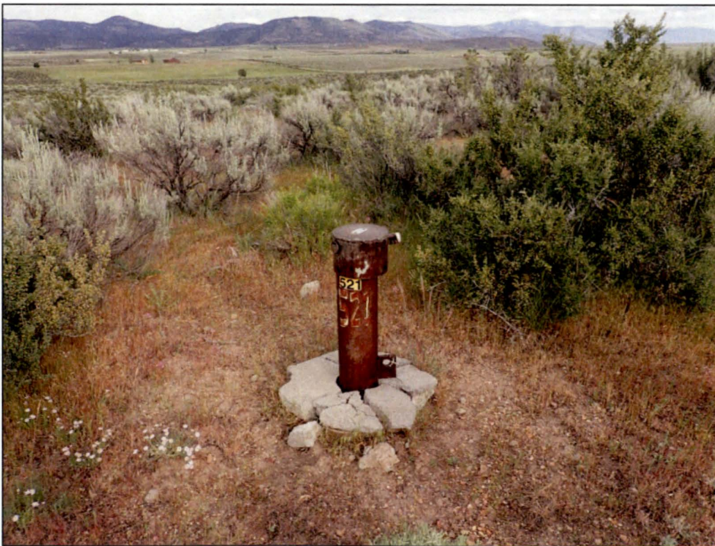
PL-8. Monitoring Well 0521 with Cracked Concrete Base
