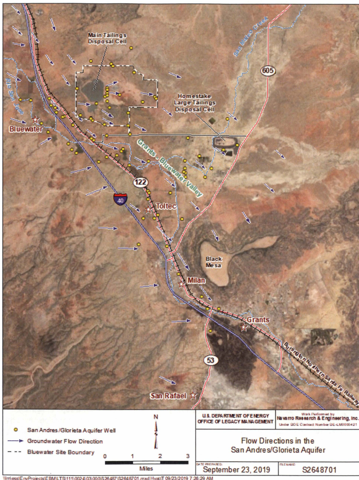
Figure 1-6. Groundwater Flow Directions in the San Andres/Glorieta Aquifer at the Bluewater, New Mexico, Disposal Site
