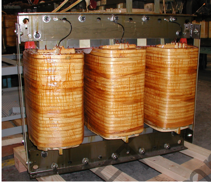
Figure 5-17 Example of Typical Dry-Type Transformer Internal Winding Assembly
