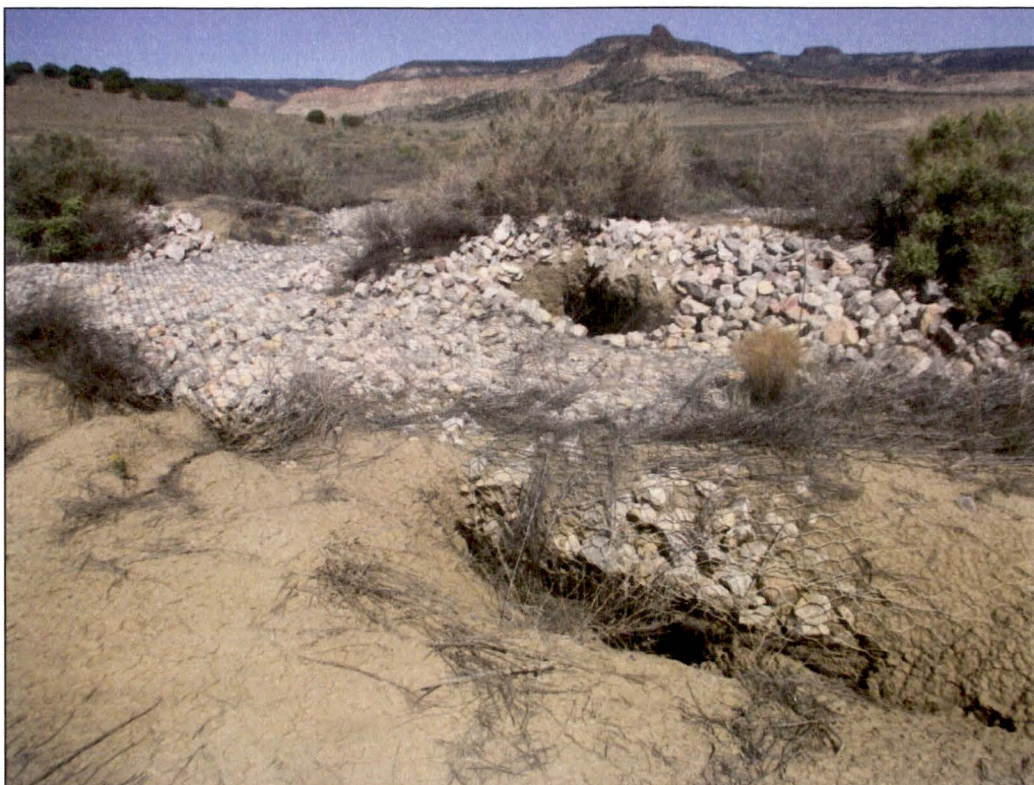
PL-13. Soil Piping Along Inlet of Runoff Control Structure A
