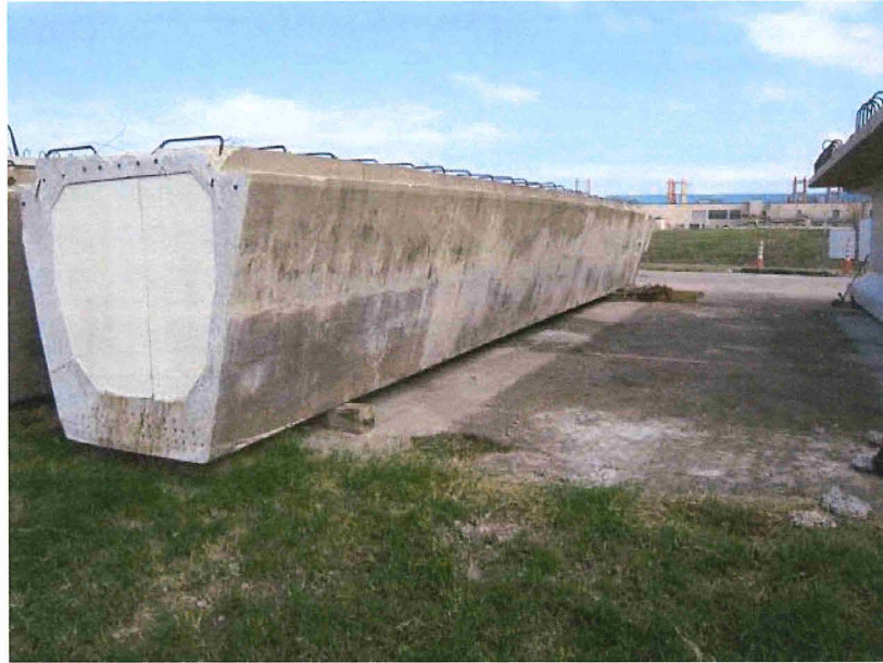
Figure A-1. Photo of Girder Series Anchor Test Specimen
