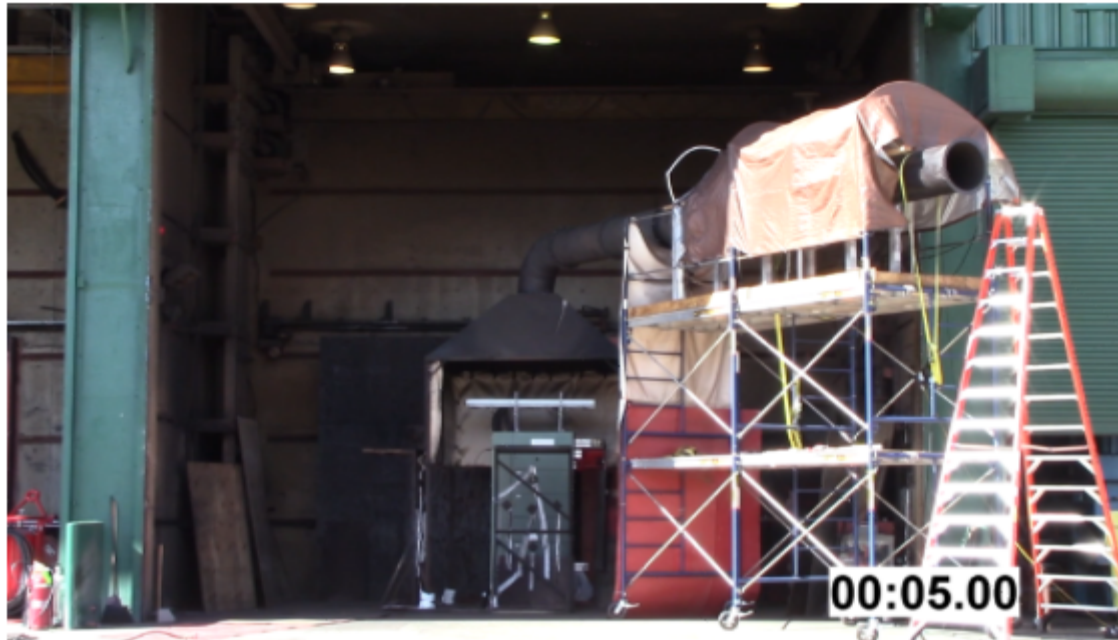
Test #23: 480 V, 40 kA, 7 seconds Aluminum bus bars
