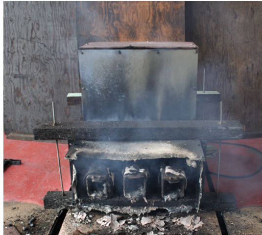
Zion Bus Duct (testing) 2016
