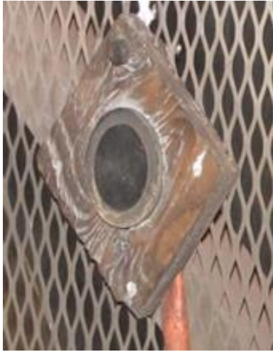
Figure 8. Slug calorimeter installed on a test stand.
