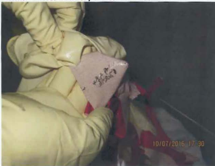
Material removed from body of check valve BG8497
