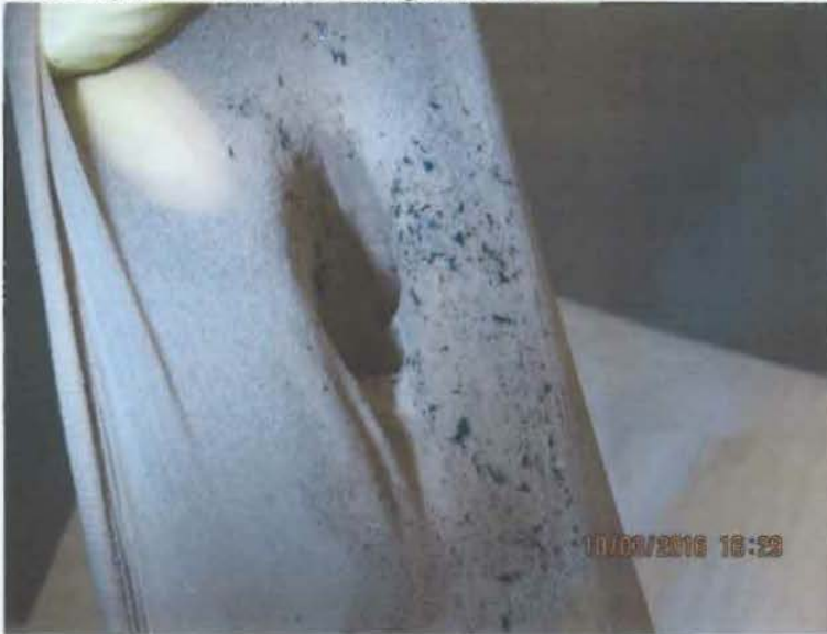
BGV0821, NCP Balance Line Casing Drain debris
