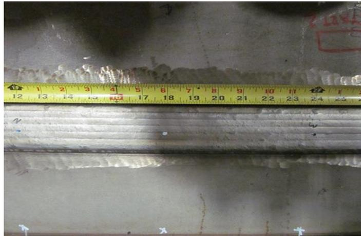
Initial weld on plate specimen with identification of 3 sets of 10 measurements
