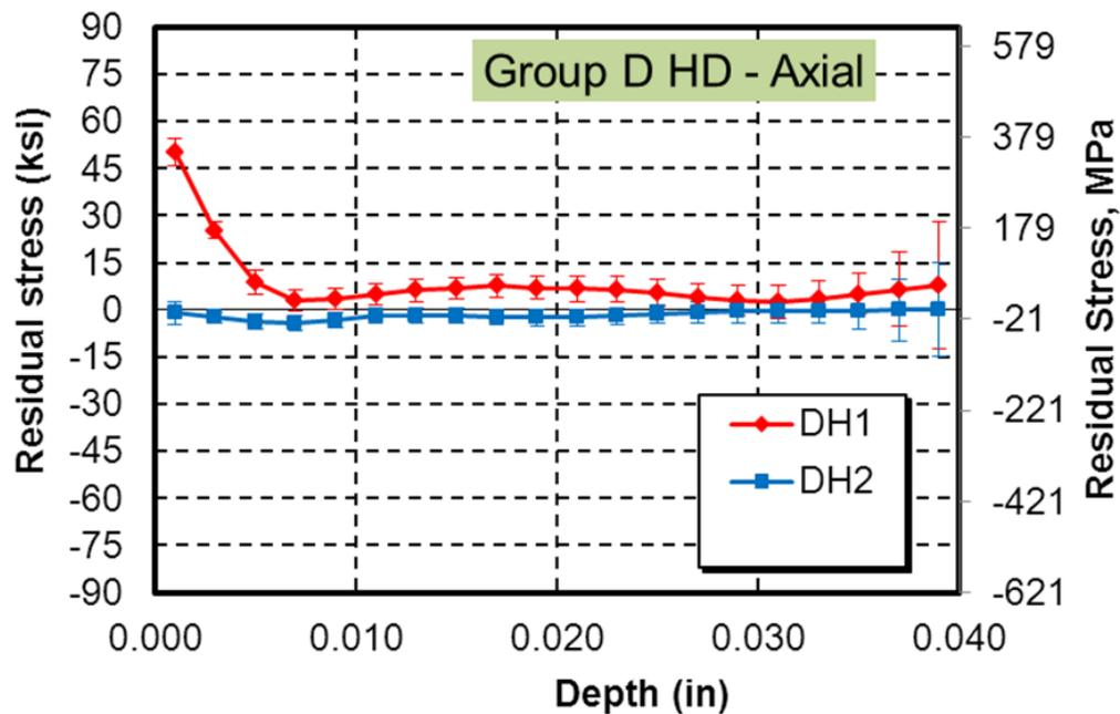
The location of these measurements was based on a generic WRS model. Both had high tensile stresses identified by the model. However, DH1 is greater than 10 ksi for only about half of the thickness and DH2 is in compression.
