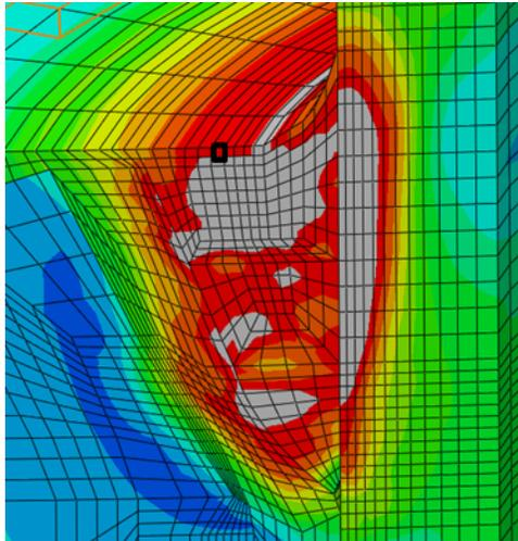
Concerns about variety of stress profiles identified may be alleviated by peening and evaluation of the final peened stresses
