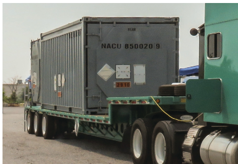
Truck carries NAC LWT transport package.
