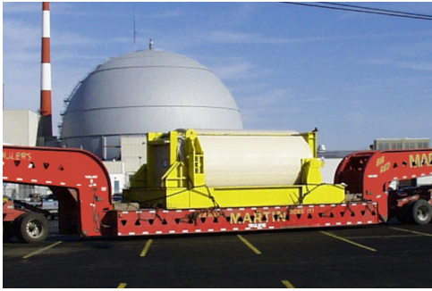
Transportable spent fuel storage cask moves to storage pad.
