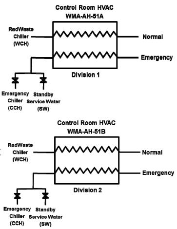
Normal cooling coil supplied by the Radwaste Chiller Water (WCH) Emergency cooling coil supplied by Standby Service Water (SW) or CCH
