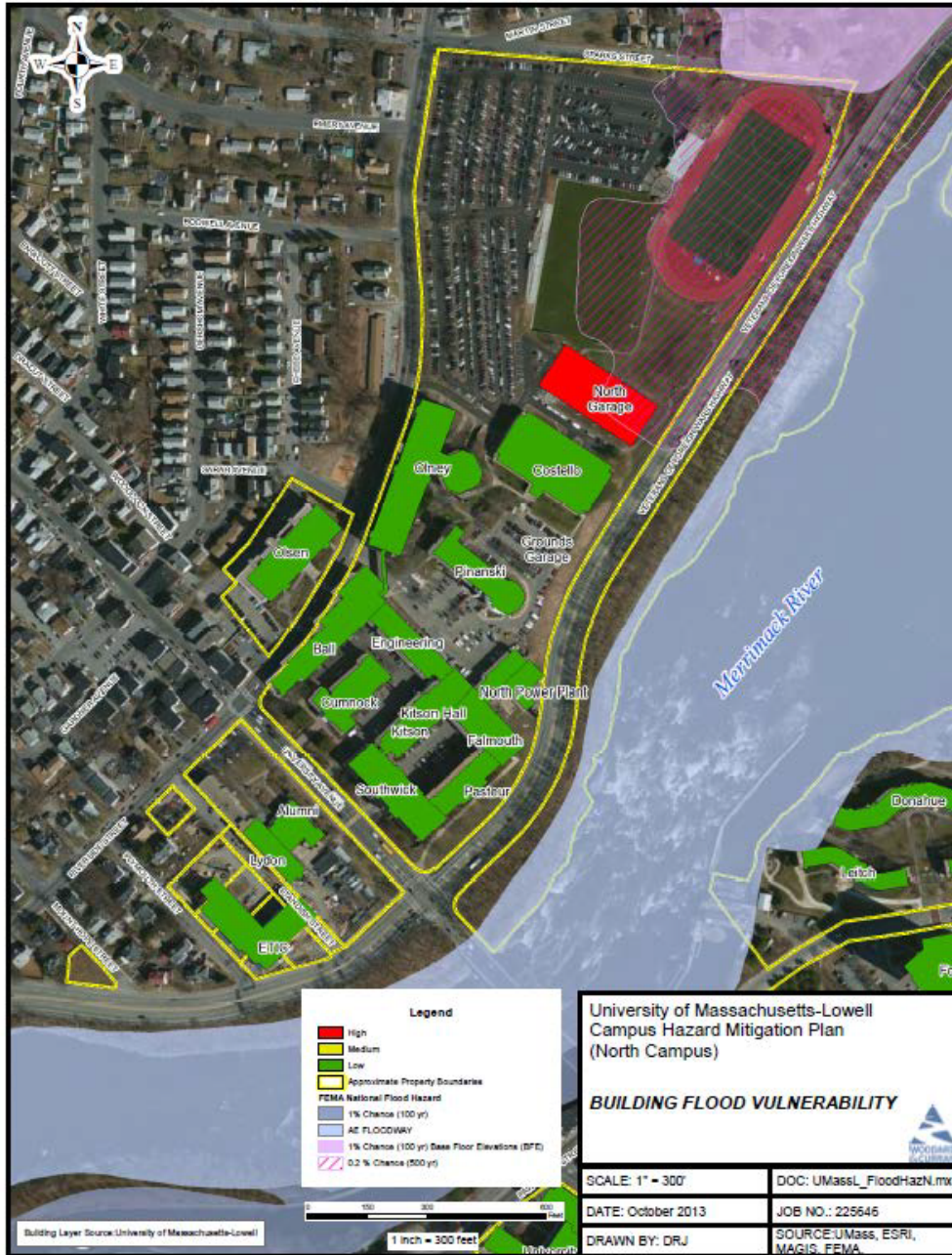
Figure 2-16: Flood Vulnerability Assessment – North Campus (Mitigation Plan)
