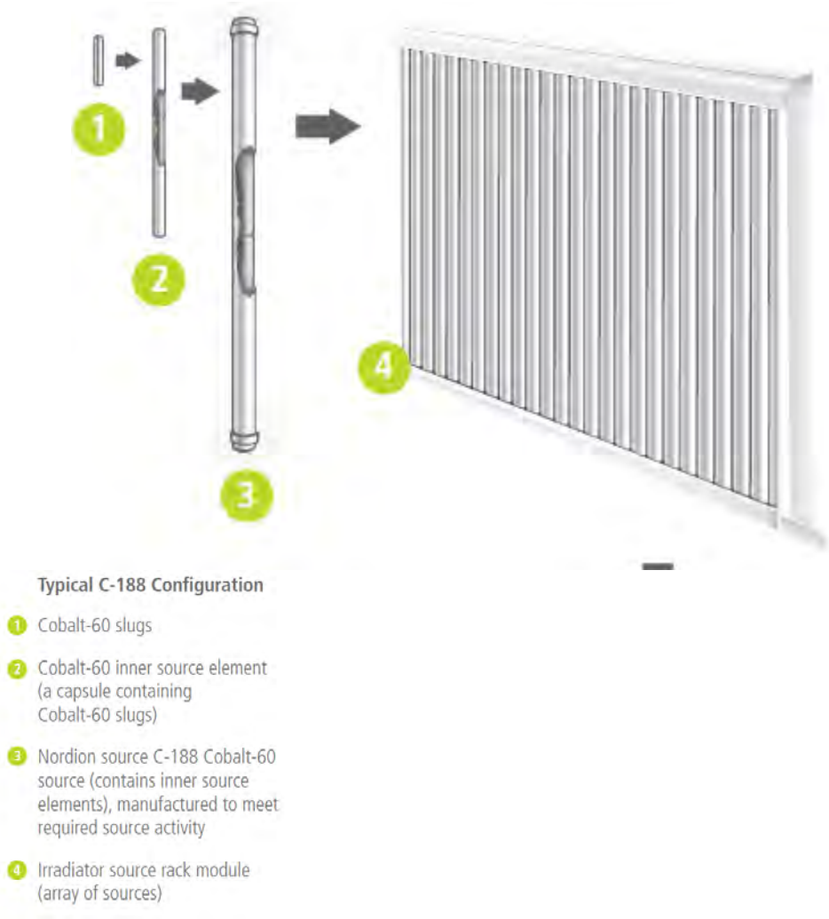
Figure 10-6: Cobalt-60 Sources and Geometry
